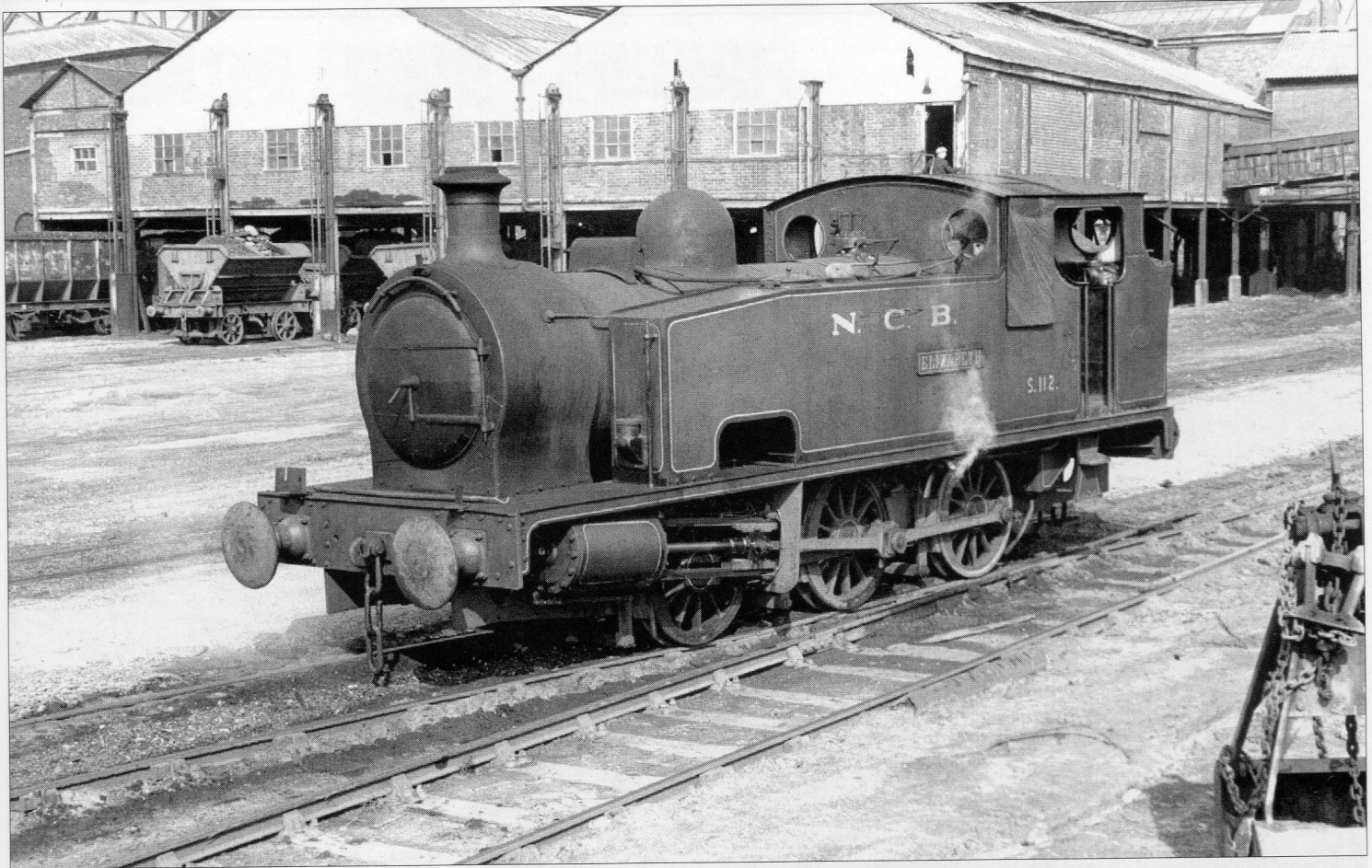
Elizabeth pauses at the east side of the screens while between duties on 11 June 1969. In the background, BR 21-ton and NCB side-tipping (Jubilee) wagons are being loaded at the screens. The Jubilees were usually loaded at the washery, so their presence at the screens indicates that they were about to be loaded with muck and stone which had been excavated while driving headings and roadways underground. The screen roads were (from left to right): 1 - cobbles; 2 - Beeston seam best coal; 3-6 - 'kitchen coal'. 7 and 8 were never used. Note the ropes and pulleys on the front of the screens - these were used to counterbalance the conveyor belts from which the wagons were loaded. PHOTOGRAPH: PETER STAMPER
