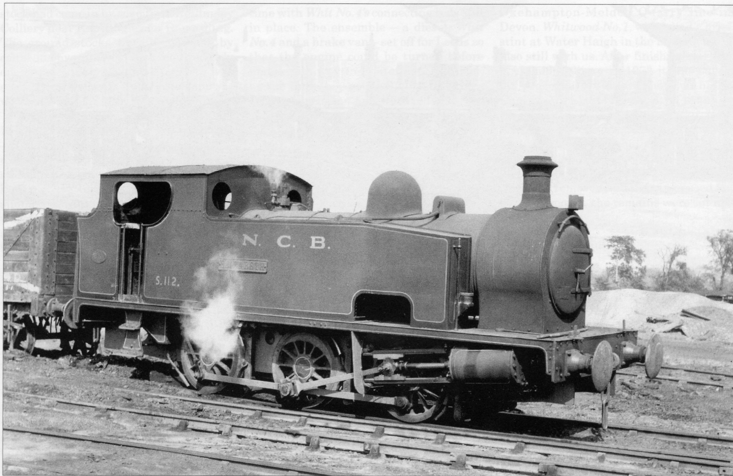
A fine portrait of the impressively-clean Elizabeth at Water Haigh on 27 August 1965. As can be seen the engine had top feed – this was a very unusual fitment for an industrial loco. PHOTOGRAPH: ROGER MONK
